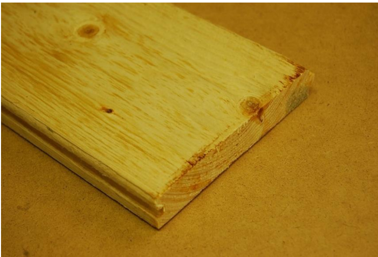
FIGURE. Cladding board made by hot pressing in Koivukunnas's tests (22 x 155 -> 20 x 150).
